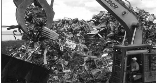
The crushed cans and cars are then picked up by a machine and put through a shredder. The shredder cuts them into tiny bits of metal.
