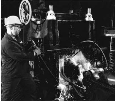
The long blocks are then heated and rolled into long thin rods.
